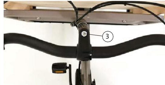
Adjusting the handlebar stem
