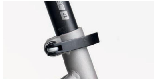
Quick release in closed position
