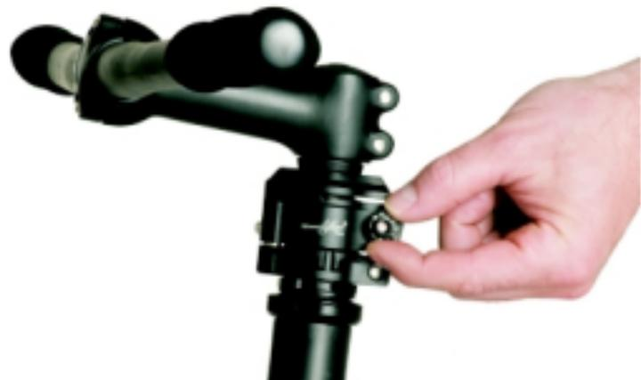
Open the quick-release lever completely. Turn the adjustment bolt clockwise a half turn and close the lever securely. Check the stability of the stem and handlebars. Should they still slide downward, this procedure must be repeated. If the lever cannot be closed completely, the adjustment bolt must be turned counter-clockwise.
