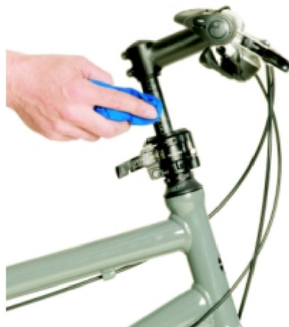
The Speedlifter systems should be maintained regularly to insure they work properly. Be sure to regularly remove any dirt from the Speedlifter. Use only water and a clean rag. If required, apply some spray-lubricant to the extension-tube and the pivot-point of the quick-release lever.
