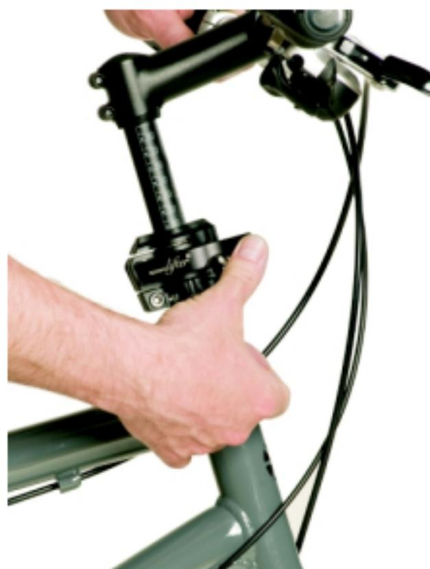
Please make absolutely sure that the Speedlifter's quick-release lever is properly closed before you ride your bicycle! Likewise the Speedlifter Twist's safety bolt must be locked into the hole at the front of the body. Be sure to check whether the operating-lever is completely closed before each trip! Never adjust handlebar height while riding! Always stop the bicycle before adjusting handlebar height!
