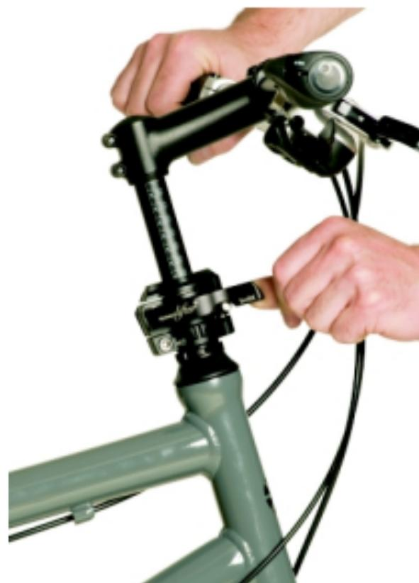
Open the Speedlifter quick-release lever by hand and adjust the height of the stem and handlebars to the desired position. Then simply close the operating-lever to lock the handlebars securely into place. It's that easy!
